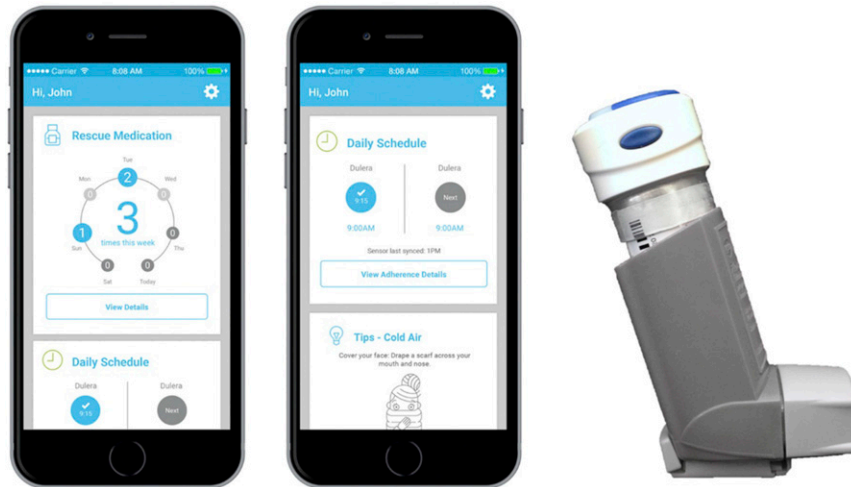
SUPPLEMENTAL FIGURE 9 Propeller sensor and cell phone application.
